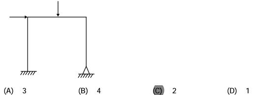
244. If only a beam mechanism is possible in the frame given below, what will be the plastic moment M<sub>n</sub> developed?
