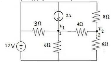
$$A = \frac{V_2 - V_1}{4} + \frac{V_2}{8} = \frac{V_2}{6}$$
