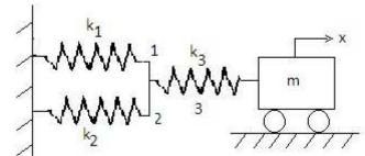
Which one of the following is the correct value of the natural frequency (  $\omega_n$ ) of the system given above ?
