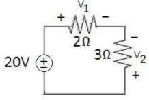
$$|V_1 = 8V, V_2 = 12V$$
