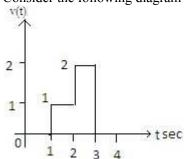
Which one of the following gives Laplace transform of the voltage v(t) shown in the above diagram?
