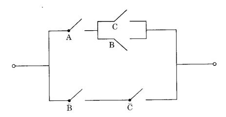
Determine the Boolean expression corresponding to the switching circuit in the given figure.
